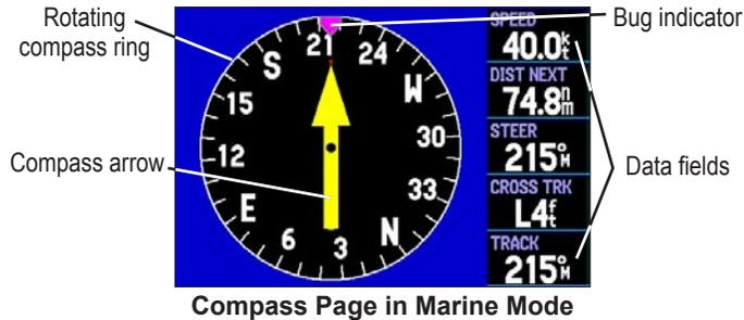
The middle of the page features a rotating compass ring that shows your course over ground (track) while you are moving. Your present course over ground is indicated at the top of the compass ring. The direction of the destination (bearing) relative to the course over ground is indicated by an arrow in the middle of the compass ring and a course to steer “bug” on the outside of the compass ring.
