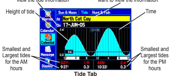
The top of the page shows the tide station and date being referenced. The chart shows a 24-hour block of time, with the time progressing from left to right. The solid vertical lines represent 4-hour increments; the dotted vertical lines represent 1-hour increments.
