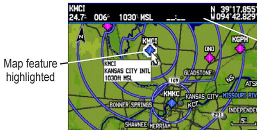
Panning Arrow data window: shows the distance and bearing from your present location, feature's elevation, time to the feature, and arrow's location coordinates.
