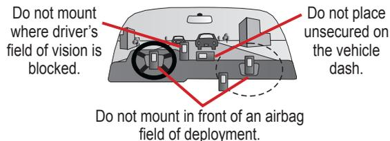
Always operate the vehicle in a safe manner. Do not become distracted by the GPSMAP 296 while driving, and always be fully aware of all driving conditions. Minimize the amount of time spent viewing the screen of the GPSMAP 296 while driving and use voice prompts when possible. Do not enter destinations, change settings, or access any functions requiring prolonged use of the unit's controls while driving. Pull over in a safe and legal manner before attempting such operations.
